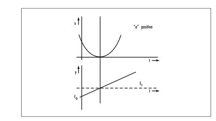
Figure A2. Positive Frequency Drift
