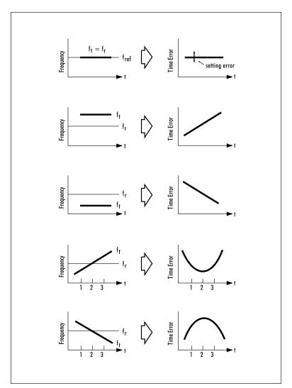
Figure A4 shows corresponding plots of frequency and time errors to clarify their relationship.
