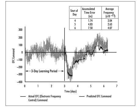
Figure 8. Example of holdover showing environmental effects.
