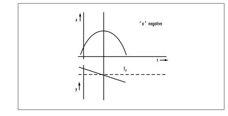
Figure A3. Negative Frequency Drift
