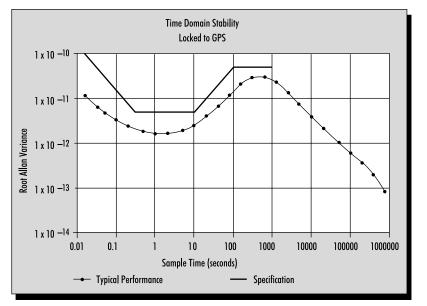
Figure 6. Root Allan Variance of the SA filtered time difference data measured by a 58503B GPS Time and Frequency Reference Receiver.
